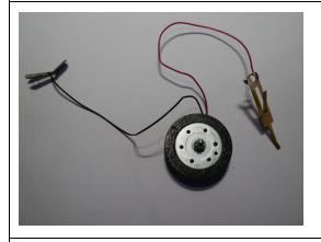
Next, the motor ring adaptor (large deep ring) needs to be fitted to the new motor and original bogie contacts soldered to the motor cables.
