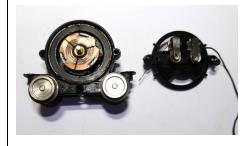
There are two small screws either side of the brush holder, once these are removed the brush holder can be removed and placed to one side, this will no longer be needed, but keep the screws safe as these will be reused.
