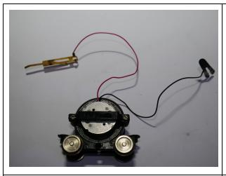
The final stage is to insert the new motor and ring adaptor to the original bogie casing. This will push fit into location. It is best to point the wires up and out of the way of the moving parts etc.
